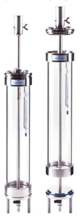
The Standard Water Sampler (whilst open) is lowered into the water by rope. Upon reaching the desired depth, the messenger activated closing mechanism is released and closes the lids of the sampling tube. A built-in thermometer, ranging from  $-2^{\circ}$ to  $+30^{\circ}$ C, indicates the temperature of the sample. To retrieve the water sample for analyses only the discharge cock at the lower lid has to be opened.
